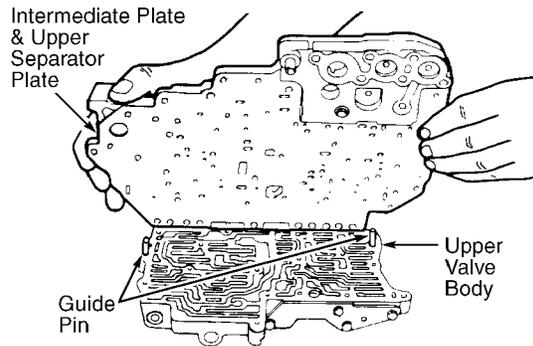
INSTALLING GUIDE PINS IN UPPER VALVE BODY
