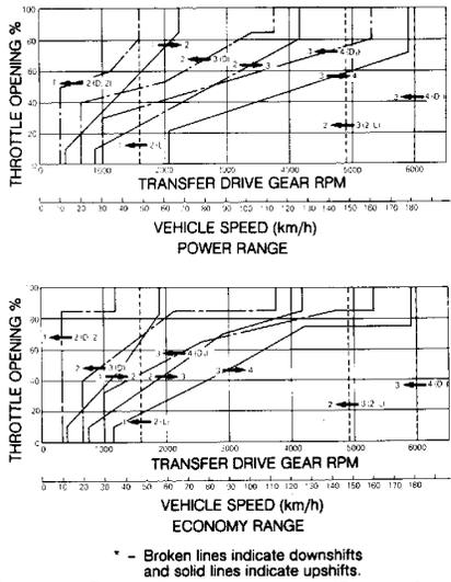
Fig. 6: Identifying Transaxle Shift Points (3000 GT DOHC)
