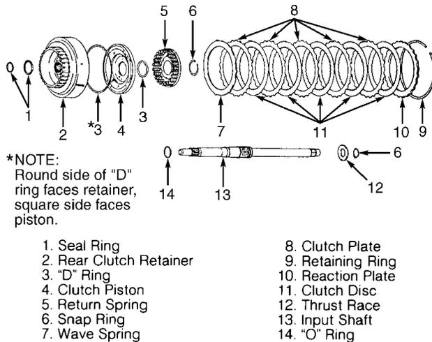
NOTE: W4A32 contains 3 clutch discs and 2 clutch plates.
