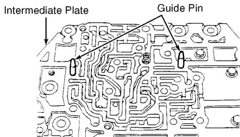
INSTALLING GUIDE PINS IN INTERMEDIATE PLATE
